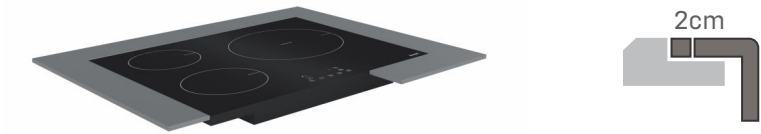
It is recommended to leave always at least 2mm between the fixtures and the edge of the cutout.
